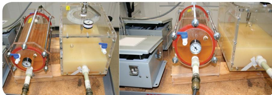
**FIGURE 1** The setup for corrosion tests on steel LPR and ER probes using 10% VCI and nitrogen blanketing at 10 psi applied pressure.
