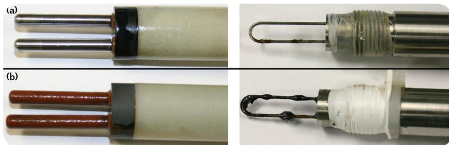
**FIGURE 4** Comparison of corrosion damages on both LPR and ER probes (1020 steel) in (a) VCI and (b) nitrogen blanketing system.
