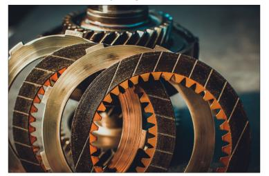
mild enough, to perform rust removal in 10-20 minutes without hydrogen embrittlement. It took about nine months to complete rust removal on all 1.7 million parts, but the clutch plates were finally restored, neutralized, and packaged for a huge savings to the automaker.
