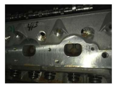
would meet GM specs for testing in humidity and salt spray conditions. EcoLine<sup>®</sup> 3690 was one of the two products tested and proved to be the more effective choice. The product met GM specs, whereupon EcoLine<sup>®</sup> 3690 was adopted for long-term indoor storage of all-time-buys (up to 10 years' build-ahead of new parts) including crankshafts, camshafts, and cylinder heads.
