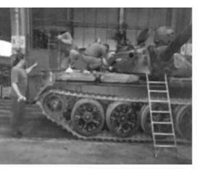
The Croatian Army was looking for solutions to remedy corrosion problems out in the field. These problems were hindering immediate combat readiness. Their tanks were especially affected by the corrosion in several areas throughout the country. VpCI®-325 was used to protect all shafts bearings, machined surfaces and other unpainted internal surfaces.
