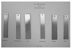
Specimens that were immersed in VpCI-325, after 1 week. All specimens display no corrosion.
