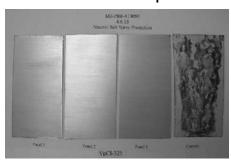
VpCI-325 on 7075-T6 Aluminum panels after 336 hours, no corrosion is seen on the panels coated with VpCI-325.
