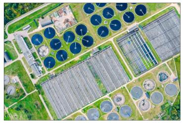
Wastewater treatment plants rely on naturally occurring microorganisms to break down waste substances. Practically speaking, the microorganisms feed on the waste and eliminate it from water and/or convert toxins into harmless substances that can be safely discharged back to the environment. However, this delicate
