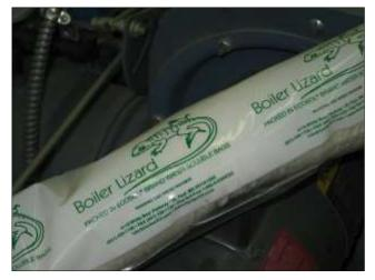
Boiler Lizard<sup>®</sup> contains Vapor phase Corrosion Inhibitor powder in a polyvinyl alcohol (PVA) watersoluble bag. The powder formulation is free of phosphates, heavy metals, nitrites, and free amines. Designed for dry layup of boilers and other boiler systems, the Boiler Lizard<sup>®</sup> protects metals in enclosed spaces by emitting Vapor phase Corrosion Inhibitors that adsorb as a protective molecular layer on all metal surfaces, reaching recessed areas and interior cavities.
