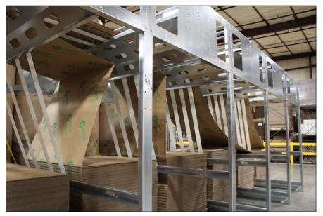
Cortec<sup>®</sup> is the first company to get this upgraded model of on-demand box maker, which draws from six stacks of fanfold cardboard. The machine cuts, scores, and glues the cardboard so it can be folded into boxes of different shapes and sizes. A touchscreen allows CCP to easily select box style and dimensions and switch from one type of box to another for excellent flexibility and
