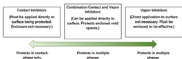
Figure 1. Corrosion inhibitors are available on a continuum ranging from contact-only inhibitors to vapour corrosion inhibitors for void spaces.
