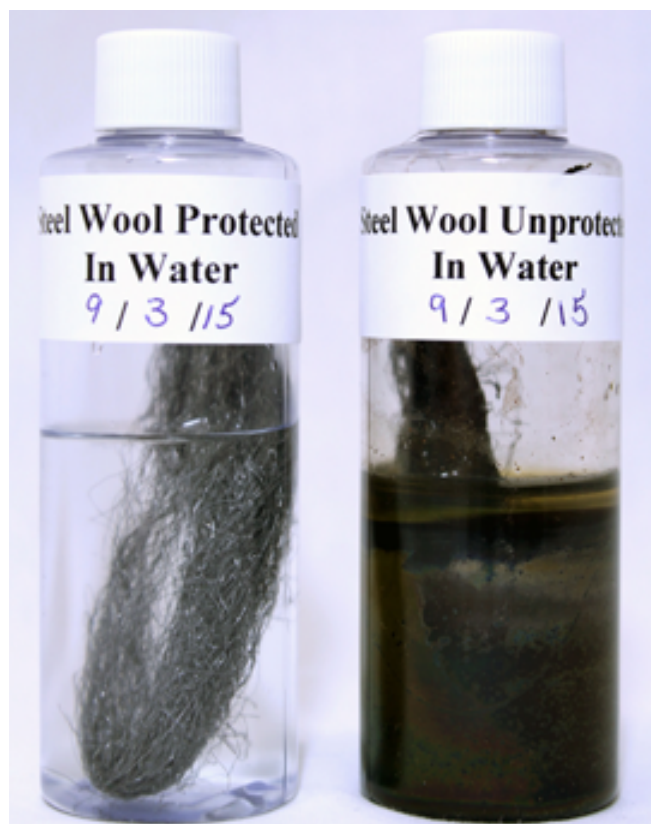
Figure 2. Left: The multi-phase action of VCIs protects the steel wool below the surface of the water, above the surface of the water, and at the air/water interface. Right: Steel wool in the bottle is not protected.
