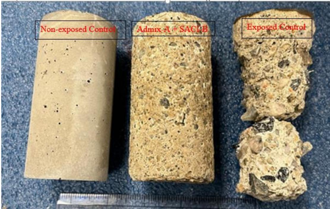
Figure 5: The exposed surface conditions for concrete samples after 400 days of immersion. Control and Concrete + 5.0%Admix-A + SACI-B in pH 2.2 solution+300 ppm sulfide. The control concrete sample showed severe sulfate attacks while combination of Admix-A+SACI-B showed no sign of any surface corrosion attacks.
