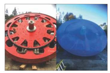
lar layer on all metal surfaces inside an enclosed package. When the component reaches its destination, it can simply be unwrapped and used immediately without additional cleaning or degreasing. This is unlike many traditional methods, such as those in the auto industry, where parts are often dipped in petroleumbased rust preventatives that
