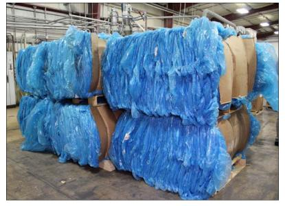
Recycling is nothing new at CAF, where recycling and reprocessing of film scrap has been going on for decades. With the installation of state-of-the-art reprocessing equipment, CAF ramped up its capabilities when it moved reprocessing in house. CAF incorporates the "repro" back into the virgin film at up to 20 percent, a level at which CAF can ensure quality of the new product. "Almost nothing goes in the
