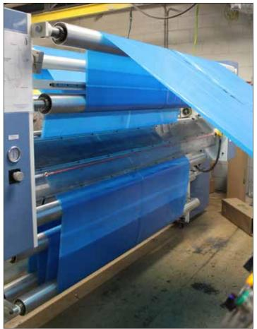
In addition to providing more versatile options for protecting large equipment from corrosion, this wide format also increases production capacity. Recent output was as much as 1700 pounds (771 kg) an hour, and the future goal is to reach 2,000 pounds (907 kg) an hour. With these new efficiency capabilities, CAF is eager to provide more service to the large format film market.
