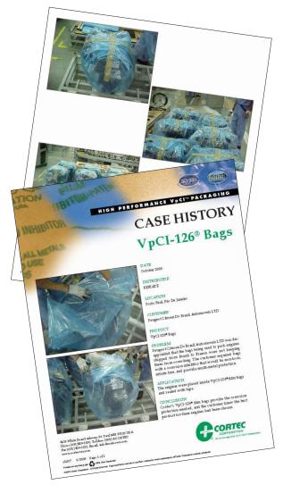
A Brazilian automotive manufacturer was disappointed when the bags they used to package engines for shipment from Brazil to France failed to stop corrosion. The customer wanted a multi-metal protection solution involving nitrate-free bags that would be safe for users to handle.
