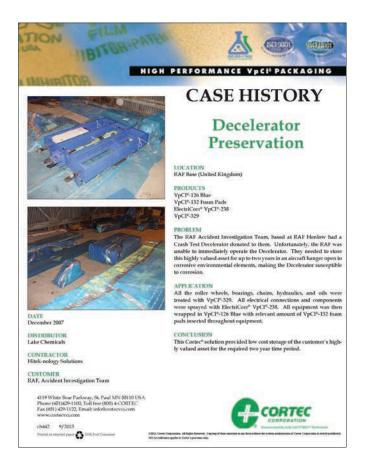
An air force accident investigation team in Europe received a donated crash test decelerator that they were not able to start using right away. Instead, they had to store this high value asset for up to two years in an aircraft hangar open to corrosive environmental elements.
