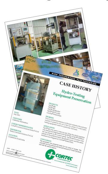
A perceived auto industry recession prompted a customer to put costly hydro-testing equipment into preservation. Existing rust was removed with VpCI®-426, and the machine was cleaned/degreased with VpCI®-419. A VpCI®-105 emitter was stuck inside the control panel, and VpCI®-609 pouches were placed below the electric motor. The entire machine was wrapped in Cor-Pak® Stretch Film ready for two years of storage to the customer's satisfaction.
