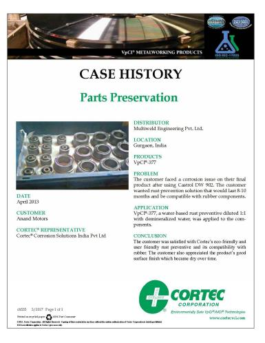
A manufacturer was having corrosion issues on finished metal components after using a conventional oily rust preventative. Needing a replacement that would be compatible with rubber, the manufacturer adopted VpCI®-377 water-based rust preventative, applying it at a 1:1 dilution with demineralized water. The manufacturer was satisfied with VpCI®-377 and its compatibility to rubber components and also liked the good VpCI®-377 surface finish that dried over time.
