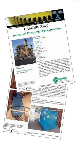
The shutdown of a natural gas fired power plant required the preservation of several costly assets. These included turbines, valves and moving parts, oil tanks, adjacent equipment, and water/steam tanks. The combined internal volume of the oil systems needing protection was 13,845 gallons (52,409 L), while that of the water/steam vessels was 11,700 cubic feet (331 m³).
