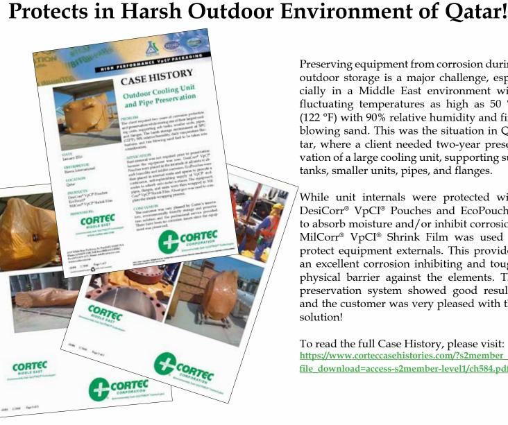
Preserving equipment from corrosion during outdoor storage is a major challenge, especially in a Middle East environment with fluctuating temperatures as high as 50 °C (122 °F) with 90% relative humidity and fine blowing sand. This was the situation in Qatar, where a client needed two-year preservation of a large cooling unit, supporting sub tanks, smaller units, pipes, and flanges.
