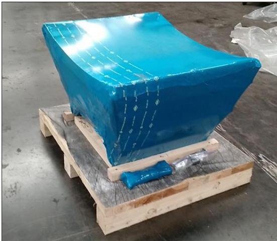
One mining equipment company with a location in Chile found components that were already showing signs of corrosion after one year of storage inside vacuum-sealed packages. The company needed to store the components corrosion-free for one more year and therefore decided to repackage the equipment in [VpCI®-126 HP UV Shrink Film](#) with [VpCI®-111 Emitters](#) inside the voids.
