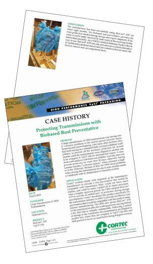
A large manufacturer of OEM transmissions was having costly problems with corrosion in the interim storage period between production and export packaging. Before the transmissions could be prepared for international shipment, they had to sit for as much as nine months in a warehouse without temperature or humidity controls. The OEM's standard wash additive was not enough to inhibit flash rust for so long. Plus, the risk of corrosion was heightened during summer months.
