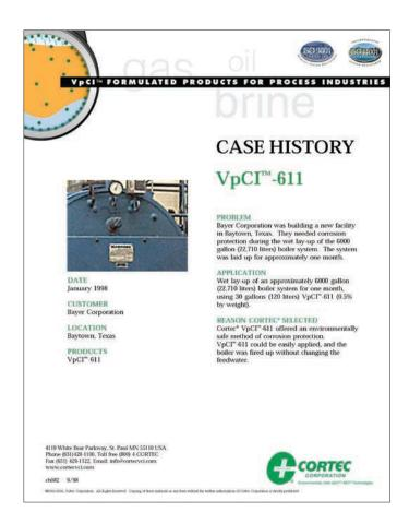
In 1998, a new facility in Texas benefited from the unique wet-layup protection of VpCI®-611, a water-based rust preventative concentrate that does not contain nitrite or phosphate. A 6,000 gallon (22,710 L) boiler at the new facility needed to be laid up wet for about one month. Thirty gallons of VpCI®-611 provided the easy to apply solution that allowed the boiler to be fired up without changing the feedwater.
