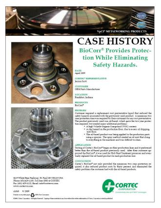
An OEM parts manufacturer needed a replacement liquid rust preventative (RP) that would provide two years of protection and reduce safety hazards posed by the previously used oil-based product. Problems with the oil-based RP included a high VOC, a slip hazard from excess oil dripping on the production floor, and an oily mist that made machine cleanup difficult.
