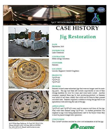
A major manufacturing conglomerate had redundant jigs that were no longer needed. Another company wanted to buy the jigs to use for manufacturing products, but the jigs were not in saleable condition. They had rusted badly during unprotected outdoor storage for more than two years. By removing rust with VpCI®-422 and VpCI®-423 and cleaning the jigs with VpCI®-416, the manufacturer was able to reclaim the jigs at low cost, then sell and ship them to the buyer ready for immediate use upon arrival.
