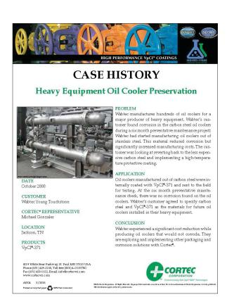
A heavy equipment producer found corrosion inside carbon steel oil coolers during a six-month preventative maintenance check. The cooler manufacturer was able to reduce corrosion by switching to stainless steel but found that this significantly increased manufacturing costs. They decided to see if they could revert to carbon steel by internally coating the coolers with a high-temperature protective coating: VpCI®-371.
