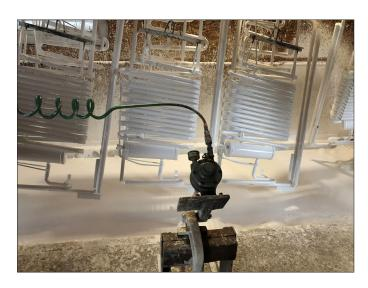
Due to the strong solvent smell, hazards, and inadequate corrosion protection of the solvent-based paint they were using, a refrigerator coil manufacturer decided to switch to <a href="VpCl®-386">VpCl®-386</a>. They kept this water-based paint in their dip tank, circulating the product to keep it mixed and covering the tank when not dipping the coils. As a result, the manufacturer was able to reduce their VOCs while also achieving superior corrosion protection.
