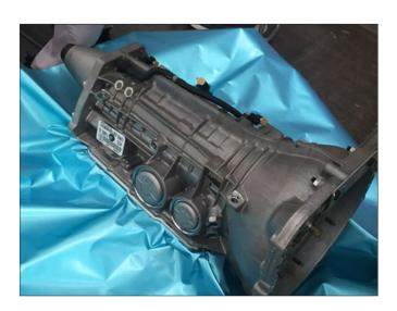
A logistics company in Thailand had 263 transmissions that it needed to store and preserve for five to seven years. They chose to wrap and seal each transmission in a piece of CorrLam® LD VpCl® Barrier Laminate. The product was easy to use and satisfactory to the customer. As of four years into the storage period, there were still no corrosion complaints!
