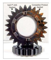
Compared to a well-known rust preventative on the market, VpCI<sup>TM</sup>-325 provides superior corrosion protection for multimetal metal parts. Test was done on a race gear, placed outdoors for 7 days
