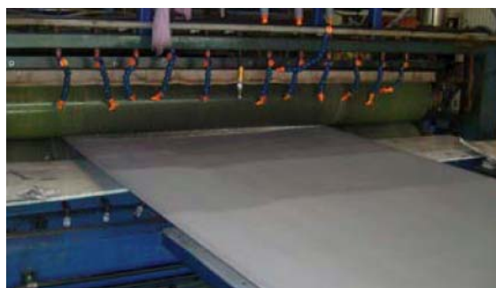
Spray application VpCI™-329D during coil processing.
