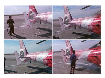
The VpCIs are built into VpCI<sup>TM</sup>-415, therefore the cleaning and rust prevention is accomplished in a single step. Once the aircraft is clean, the VpCIs protect even the smallest crevices and void spaces found on the outside skin and immediate interior surfaces susceptible to corrosive attack. Independent research tests show that VpCI<sup>TM</sup>-415 offers corrosion protection even in chloride rich environments, inhibiting pitting and stress corrosion cracking.
