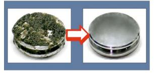
Cortec<sup>®</sup> VpCI<sup>TM</sup>-417 is especially effective for machined aluminum and magnesium castings. It removes lubricants and metal filings while providing protection against oxidation all in the same processing stage.
