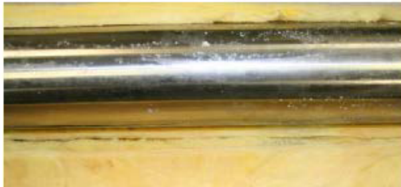
Pipe protected with VpCl®-619.
