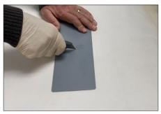
Rick also demonstrated how to do the same basic test out in the field when a kit is not available. Instead of using a special cutter, the painter can simply make two perpendicular sets of 11 cuts with a utility knife and see how many paint squares come off with a piece of tape. If the adhesion is good and few to no squares of paint come off, the coating should be cured enough to repaint!
