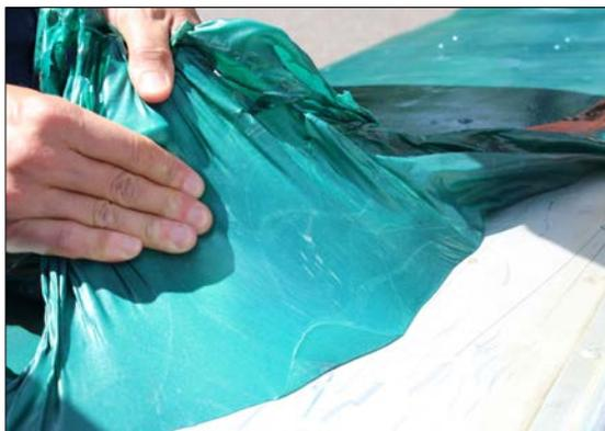
Cortec® VpCI® removable coatings are an excellent option for short- or intermediate-term corrosion protection on valuable equipment and components. They typically leave a translucent, waxy coating that cures to a soft film and eventually hardens. Variations include a thin-film water-based coating that dries clear, a heavy-duty coating for harsh outdoor applications such as offshore layup, and a peelable
