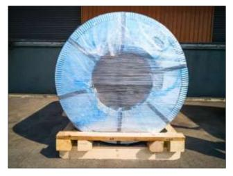
excellent packaging options that contain Vapor phase Corrosion Inhibitors right in the film, providing a physical barrier to the steel as well as proactive corrosion protection. These two films are compatible with C-hook or automatic stretch-wrapping equipment, respectively, for ease of application.
