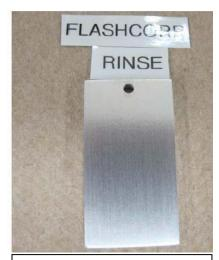
FlashCorr VpCI<sup>®</sup> protected pannel showed no corrosion after one week.
