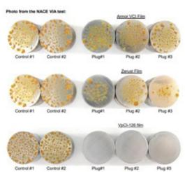
Two competitor films recently failed razor blade and VIA testing after being received in good condition at Cortec® Laboratories. The corrosion protection capabilities of the blue Armor film and yellow Zerust film samples were being evaluated on behalf of a manufacturer who used these brands and was contemplating a switch to Cortec® VpCI® film.
