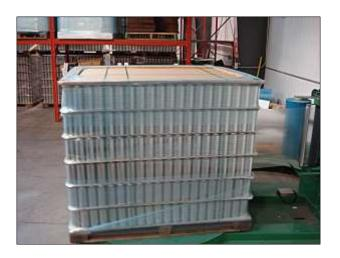
Vapor phase Corrosion Inhibitors in the stretch film do not leave residue, allowing immediate use of protected parts with no additional cleaning required.
