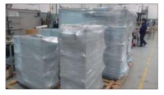
Cor-Pak® VpCI® Stretch Film is extremely convenient because it does not require users to significantly change their packaging process. This was important for a manufacturer of heat exchangers who was having trouble with corrosion on equipment being shipped overseas. Since stretch-wrapping was already part of their packaging process, it was easy to implement Cor-
