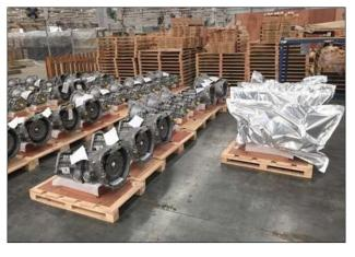
laminated to the inside of the foil releases Vapor phase Corrosion Inhibitors into the package to form an invisible molecular layer of corrosion protection that does not need to be removed from the metal component before use or further assembly. The foil prevents this molecular vapor from escaping the package, thereby trapping the protective chemistry within. Altogether, this tough, puncture- and tear-resistant packaging material is an excellent way to prevent corrosion on metal parts,
