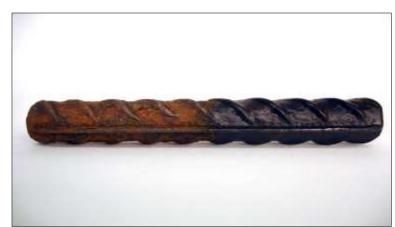
CorrVerter® eliminates the blast, passivates the rust, and leaves behind a well-primed surface with excellent adhesion.
