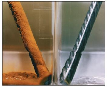
CorrVerter® works by combining a unique formulation of chelating agents with a high solids waterborne latex that has extremely low water vapor permeability. The combination of these materials modifies the surface rust into a hydrophobic passive layer, offering a unique water-based primer with excellent protection against re-rusting. CorrVerter® is recommended for application to rusty or poorly prepared steel surfaces where further corrosion protection is required, and where good surface
