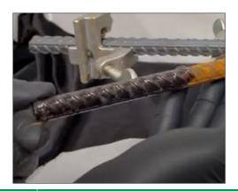
Cortec<sup>®</sup> is pleased to release a new demo video on how to apply <u>CorrVerter<sup>®</sup> MCl<sup>®</sup></u> to rusty rebar! The demo shows how to transform a piece of rusty rebar into a primed and passivated one, as required for good concrete repair surface prep. It is a great resource to share with engineers, contractors, and anyone involved in concrete construction or restoration.
