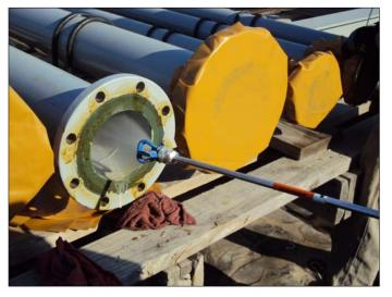
CorroLogic<sup>®</sup> Nano VpCI<sup>®</sup> Powder also has much larger specific surface area compared to larger particles of the same mass, enabling greater coverage as well as faster sublimation (transition from powder to vapor). These special physicochemical features give CorroLogic<sup>®</sup> Nano VpCI<sup>®</sup> Powder faster protection kinetics and enable a much faster buildup of a protective VpCI<sup>®</sup> environment in hard-to-reach recessed voids.
