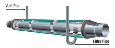
CorroLogic® VpCI® Filler was designed at the request of a North American pipeline corrosion engineering group looking for a product that would protect annular
