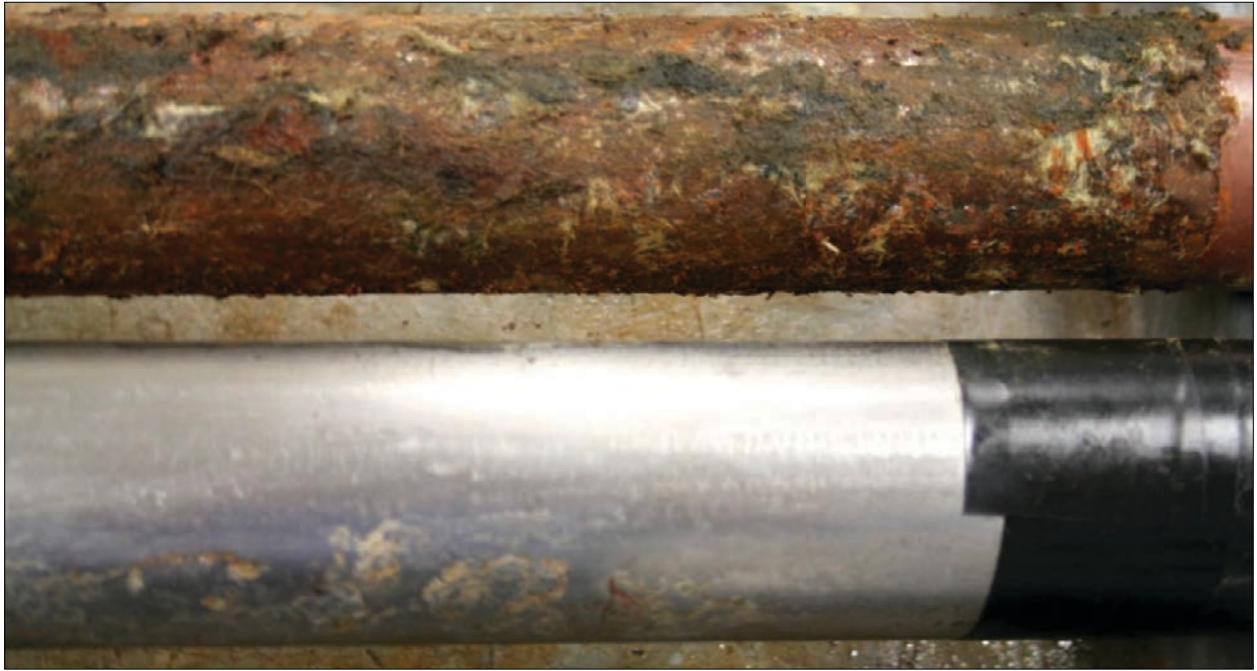
Figure 2: Pipes after 210 Days of Corrosion Testing 1 CorroLogic ® CUI Inhibitor was applied to the bottom pipe.
