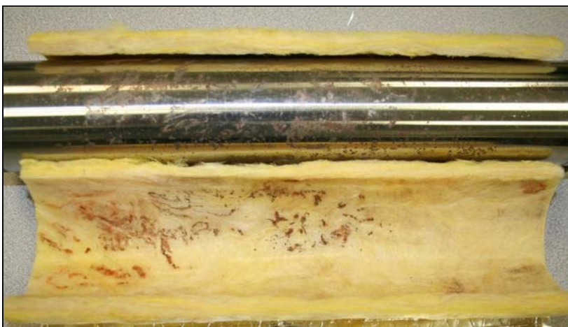
Figure 3: Unprotected pipe, after 240 hours of testing in high temperature conditions with regular chloride injection. 2
