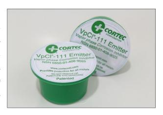
Emitters and Corrosorbers are self-adhesive cups of approximately the same size. VpCI®-111 Emitters release Vapor phase Corrosion Inhibitors through a breathable membrane, actively protecting up to 11 ft³ (0.31 m³) of space per Emitter. Corrosorber® cups absorb H<sub>2</sub>S and other corrosive gases, changing color as these gases are trapped to show when the cup needs to be replaced.
