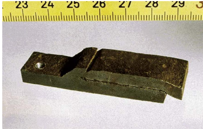
Figure 2. Bottom plate weld corrosion of crude oil storage tank after 5 years (CASE HISTORY 01.11.02.05) [8]
