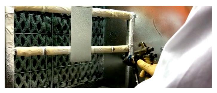
A new Cortec® video shows how to easily turn a rusted metal surface into a passivated, protected layer using CorrVerter® Rust Converter Primer!
