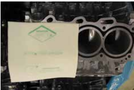
Ship's engine in Trieste, Italy, protected with VpCI foam (as marked in the picture) getting ready for ocean transport.
