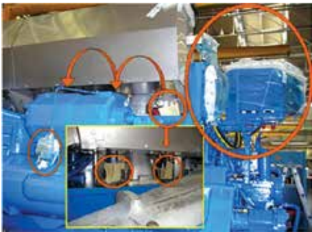
Ship's engine in Trieste, Italy, protected with VpCI foam (as marked in the picture) getting ready for ocean transport.
