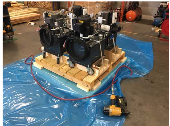
Preparing to package hydraulic power packs for a ball or SAG mill. Image courtesy: Cortec Case History 656.
