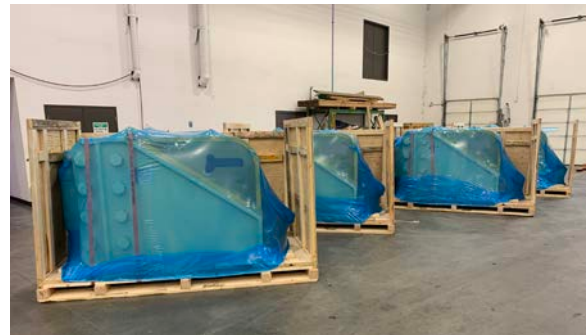
Speciality components for a ball or SAG mill packaged for shipment to South America via marine container. Image courtesy: Cortec Case History 656.
