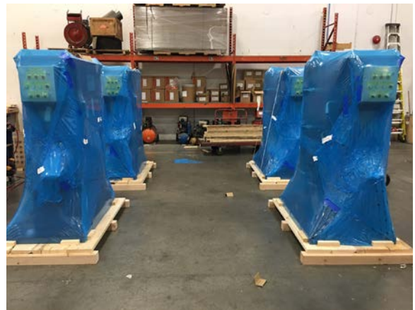
Electronic equipment shrink-wrapped in VpCI-126 for protection during shipping and storage. Image courtesy: Cortec Case History 656.
