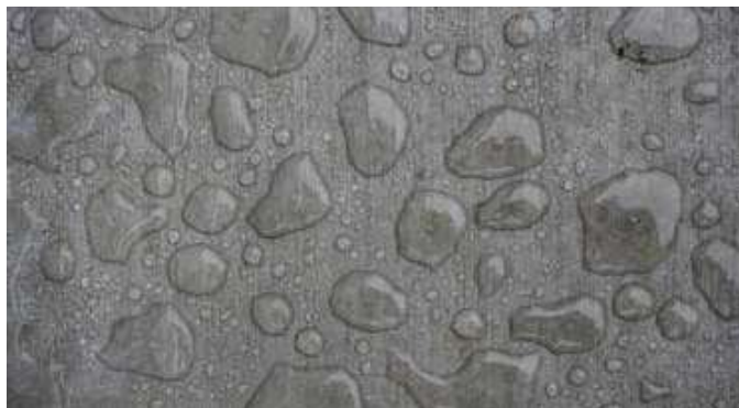
MCI-2019 seals surface pores, which prevents intrusion of chloride and carbonation and protects from the ingress of wind-driven rain
